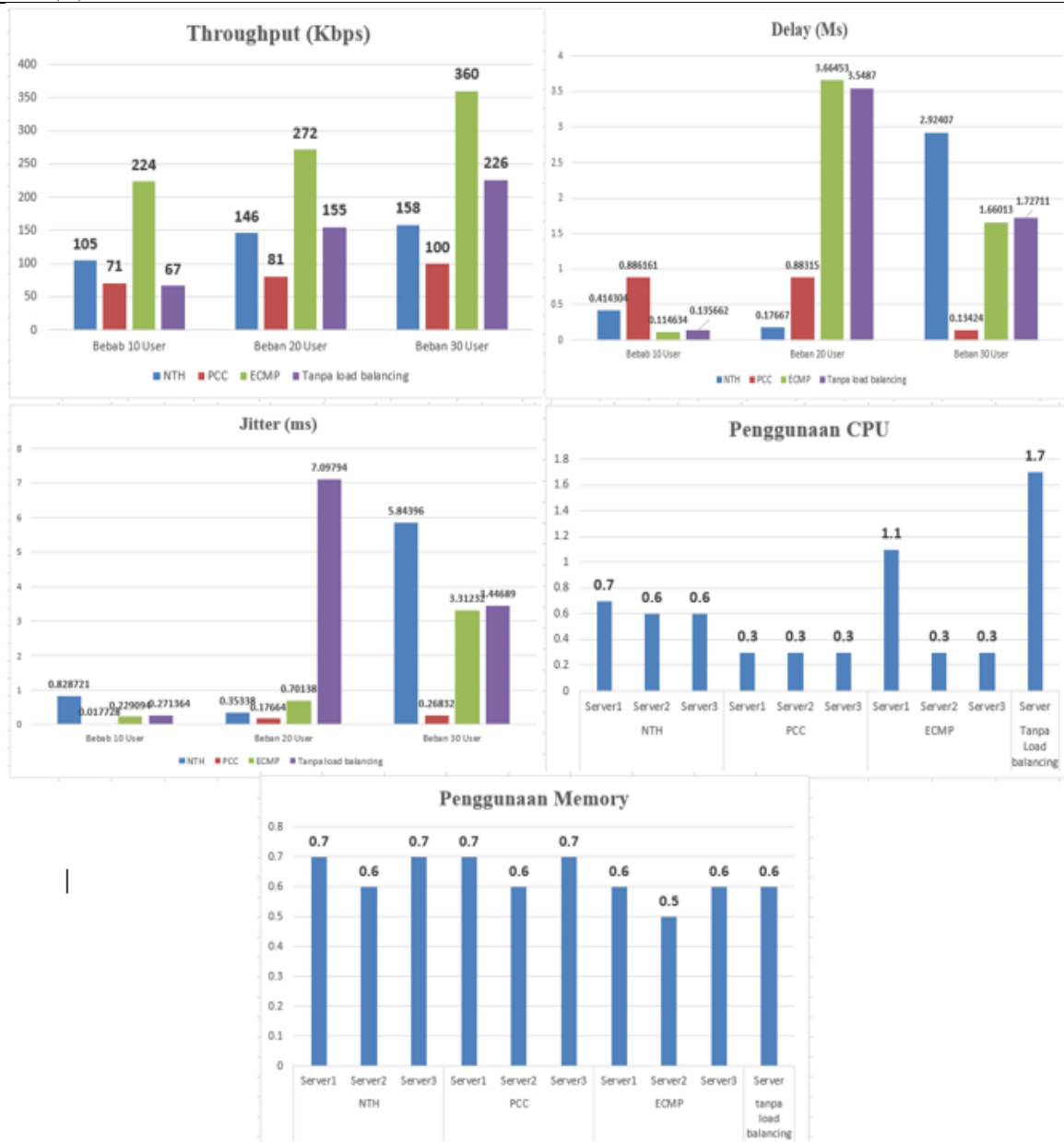
Fig 11. Results of Overall Router OS Load balancing Parameters and without Load balancing
