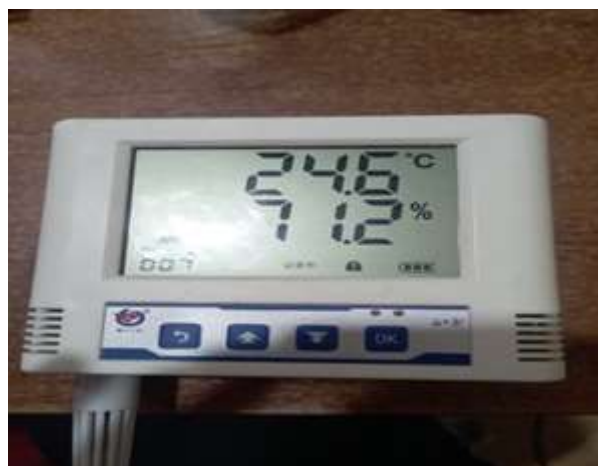
Figure 5. A-TH3 temperature and humidity sensor
