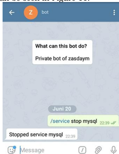
Figure 11. Service deactivation testing
