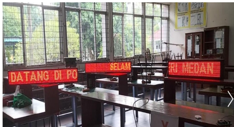
Figure 8. Testing the Running Text circuit
