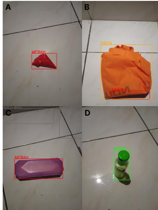
Figure 3. Screenshot of Android OpenCV for Color Detection: (A) Detecting red plastic; (B) Detecting orange tote bag; (C) Detecting purple eyeglasses case; (D) Detecting green bottle.
