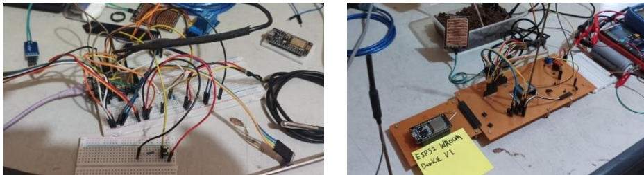
Figure 4. Monitoring System Design on Bread Board and PCB
