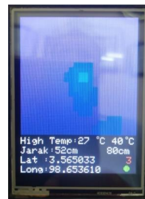
Fig 4. Testing the AMG 8833 Thermal Sensor on individual objects
