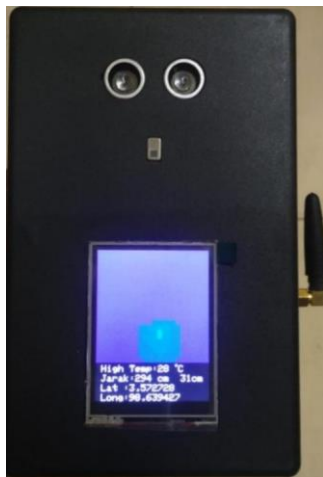
Fig 2. Prototype of Body Temperature Monitoring System
