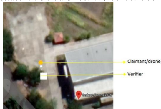
Fig 6. Authentication time testing by varying the length of random numbers under LOS conditions
