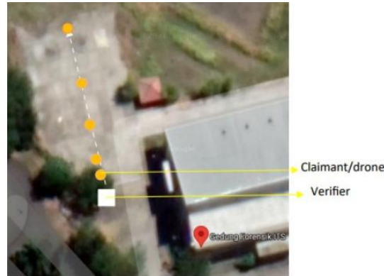
Fig 4. Testing the authentication time by varying the communication distance under conditions LOS
