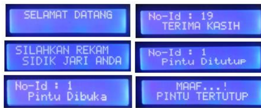
Figure 12. LCD Display When Accessing the LTK01 Room
