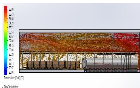
Figure 1. Heat Mapping of Sterilizer Station Side View
