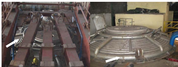
Figure 2. Roof / large lid of electric arc furnace
