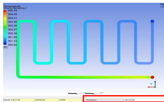
Figure 9. Maximum Temperature at Outlet
